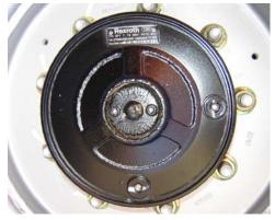
Lube Point(s) - Level/Fill Plug Capacity - 17 oz. (1/2 Full) Lube - EPGL Interval - Check level every 3 months or 150 hrs of operation; change every 2 years or 1200 hours of operation
