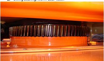
Lube Point(s) - Grease Fittings Capacity - Spray On Lube - OG or Mobiltac375NC Interval - A/R
